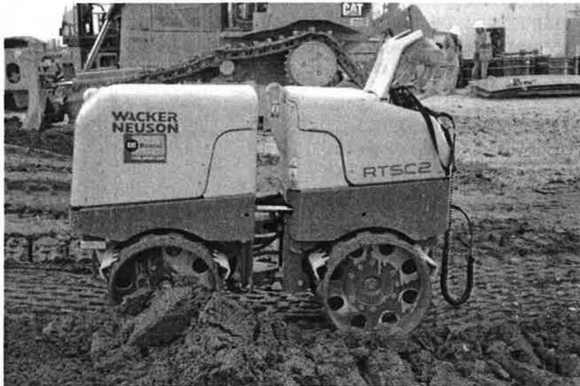
Figure 8 – Wacker Neuson RTSC2 Trench roller used for compacting north side of BAS test pad
